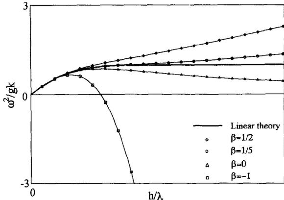
Fig. 1. Dispersion curves for various values of dispersion parameter  $\beta$  compared with linear theory.
