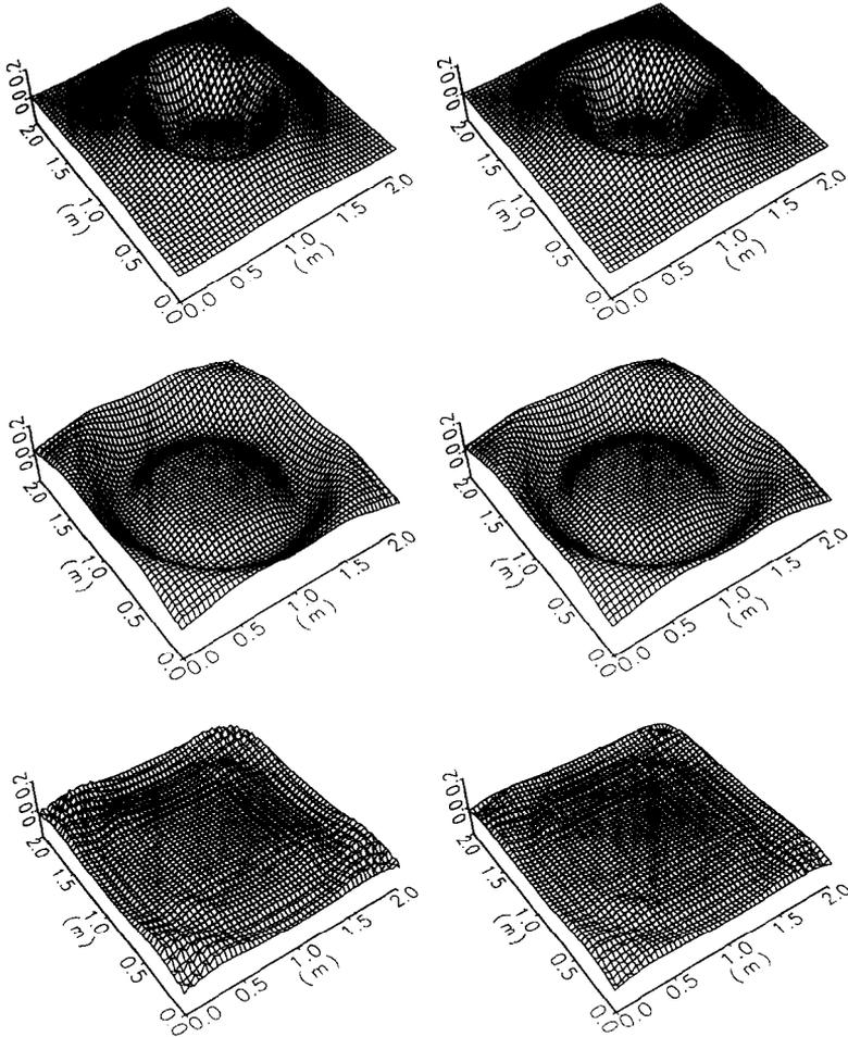
Fig. 4. Ring test displayed at  $t=1/2, 1, 2$  seconds. Left column: the first-order radiation condition, right column: the second-order radiation condition.
