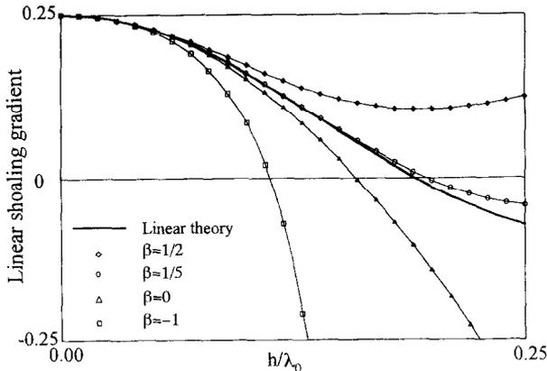
Fig. 2. Variation of the shoaling-gradient coefficient  $(c_3 - c_2c_4)/c_1$  as a function of  $h/\lambda_0$  for various values of dispersion parameter  $\beta$  compared with the expression according to linear theory.
