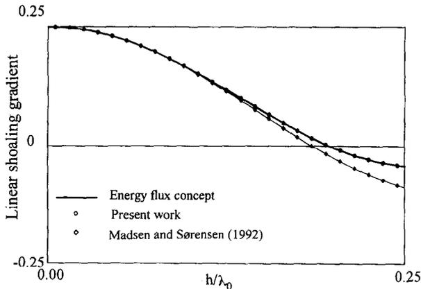
Fig. 3. Variation of the shoaling-gradient coefficient of the present work and of Madsen and Sørensen (1992) compared with the expression obtained from the energy flux concept.
