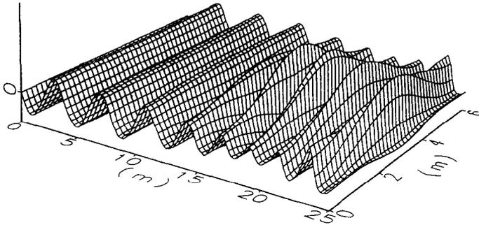
Fig. 6. A perspective view of the fully-developed wave field for incident waves of  $T=2$  seconds. Corresponds to Figure 5b.
