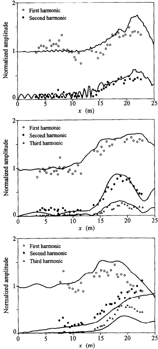
Fig. 5. a. Whalin's (1971) test for incident waves of  $T=1$  second. Measured and computed wave amplitudes along the centerline of the wave tank. Solid line: computation, scatter: experimental data; b. Same as in Figure 5a but for incident waves of  $T=2$  seconds; c. Same as in Figure 5b but for incident waves of  $T=3$  seconds.
