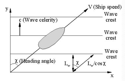
The velocity component of ship in the direction of waves is  $V \cos \chi$  and the relative speed of the ship with respect to the waves is  $c - V \cos \chi$ . Then, the time it takes the ship to travel from one crest to another is simply
